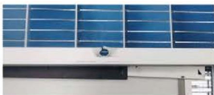
535W: torn mounting holes
